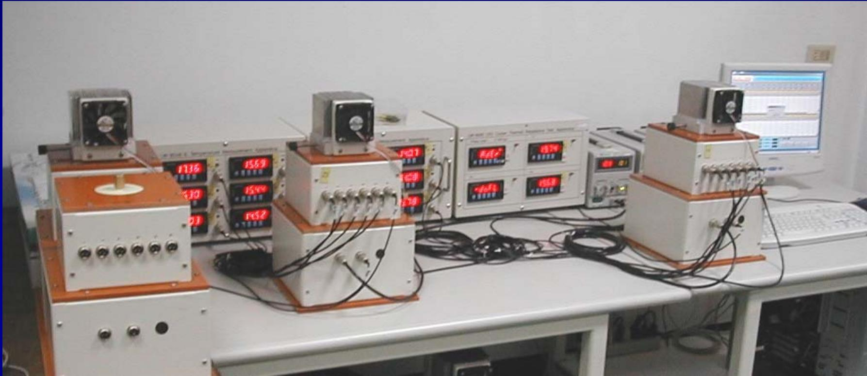
Fourier Law with ASTM-5470 D Thermal Guard concept,
