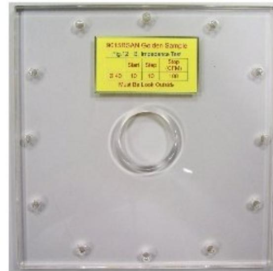
Long Win provides the orifice plate to create original flow impedance curve.
