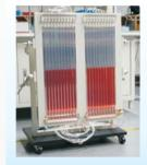
**LW-8007 Liquid manometer** Effective height: 500 mm Tube diameter 1.7 mm Inclined angle: 5 ~ 90 degree
