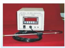
LW-9032 TSI hot wire anemometer With a digit display meter Range: 0.5~50 m/sec Accuracy: 2% of reading, or 0.5% of FS.
