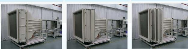
The settling section is delicately designed as a drawer type. The door is accessible for sealing up the section and open to move screen layers. Each turbulence reducing screen can be removed for cleaning.
