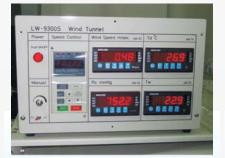
Digit meters for monitoring wind speed, atmospheric pressure and temperature.
