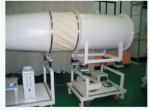
Axial Fan for driving source and canvas flexible connector for shock absorption
