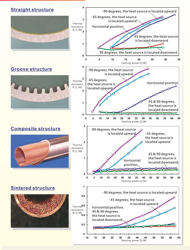
At this part, we maintain working fluid, vacancy, length, diameter, and working temperature in constant, and then compare the effect of wick structure, attitude, and heating power on heat pipes. The conclusion lists below:
