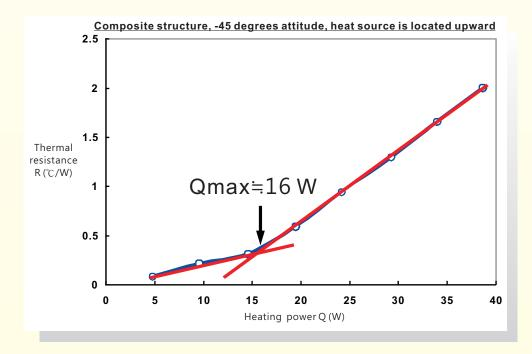
When the working fluid cannot be vaporized and recycled at a high input power, the thermal resistance will be increased suddenly.
