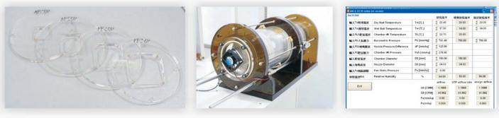
Various kinds of fixtures that can install fans with different sizes and types, It is easy to place and disassemble on the downstream of standard flow rate generator. AMCA 210 software for air flow rate calculation. Students can study the principle by using it.
