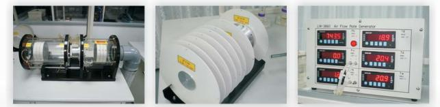
Standard flow rate generator and a set of exchangeable nozzles meeting AMCA 210-99 Standard. By cooperating with digit display meters of parameters, the system can provide a flow rate criterion in fluid mechanics laboratory.
