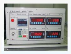
Digit meters for monitoring wind speed, atmospheric pressure and temperature.
