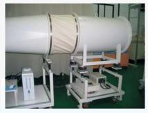
Axial Fan for driving source and canvas flexible connector for shock absorption
