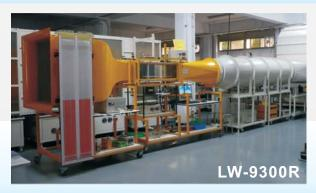
Customized wind speed range is available. In Long Win's Lab, we own a LW-9300R wind tunnel with the maximum wind speed 105 m/sec.
