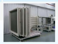
The settling section is delicately designed as a drawer type.
