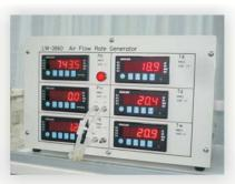
Standard flow rate generator and a set of exchangeable nozzles meeting AMCA 210-99 Standard. By cooperating with digit display meters of parameters, the system can provide a flow rate criterion in fluid mechanics laboratory.
